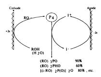
of sequential attack of nucleophilic and electrophilic components, formed respectively at the cathode and anode in undivided electrochemical cell.
